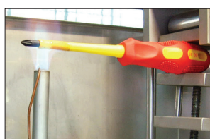
High temperature test, flame retardant test.
