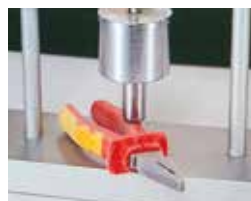
Prova alle basse temperature. Low temperature test.
