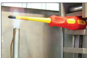
High temperature test, flame retardant test.
