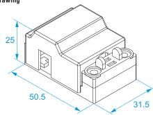
Polyamide holder with cable clamp and cover for M093 and M094 3 series
